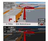
The display is adjusted using the daytime/ night-time key.
