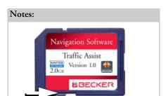
A small slider is located on one side of the card. If this is pushed in the direction of the arrow, the Memory Card is protected from being overwritten.
