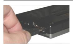
→ Use the plug to insert the mains section in the socket.
