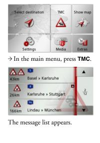
You can scroll through the list using the arrow keys **A v** on the right-hand edge of the screen.
