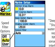
"Deep" and "Shallow" water alarms require NMEA sonar input interfacing.
