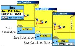
4. The Saved Track Page allows you to rename the track, view the track distance, view the calculated area encompassed by the track (an area is defined even if the track is open ended) and specify a color for the track when displayed on the map page (Show On Map). On-screen buttons at the bottom of the page allow you to save the track (OK), delete, view it on the Map, and navigate the track back to any point along the track (TracBack).
