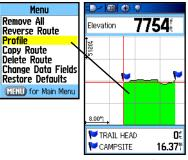
Route Vertical Profile using U.S. Topo 24K DEM mapping data
