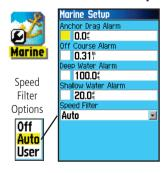
"Deep" and "Shallow" water alarms require NMEA sonar input interfacing.
