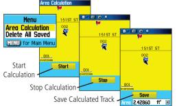
4. The Saved Track Page allows you to: Rename the track, view the track distance, view the calculated area encompassed by the track (an area is defined even if the track is open ended), specify a color for the track when displayed on the map page (Show On Map). On-screen buttons at the bottom of the page allow you to Save the track (OK), Delete, View it on the Map, and navigate the track back to any point along the track (TracBack).
