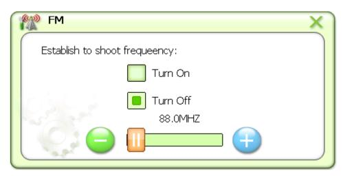
You can set "FM transmitter frequency" to "on" or "off", click" " and " " to set transmitter frequency. After setup, click " " to exit; meanwhile, please set your car's FM transmitter frequency to a certain point, then your car's acoustics can receive the audio frequency which transmits from GPS.
