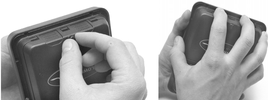
Loosen thumbscrew and remove AirMap battery cover.
