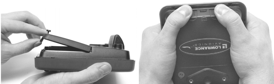
Replace battery compartment cover: Slide cover into place, left. Press in cover's bottom edge, right
