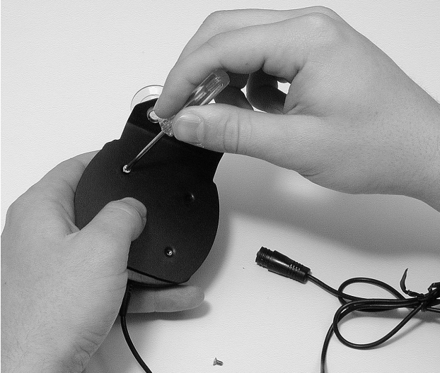
Attach AirMap antenna to windshield bracket with two screws.
