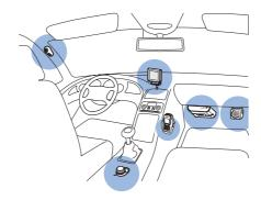
Example of appropriate installation, with the display unit mounted using the supplied adhesive
