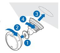
If the ambient temperature is below  $+15^{\circ}$ C (60°F), carefully warm the surface and the suction cup with a hair dryer to ensure a firm grip on the windscreen. Ensure that you do not heat the windscreen excessively to avoid damage to it.
