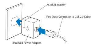
*WARNING:* Make sure the power adapter is fully assembled before plugging it into an electrical outlet.
