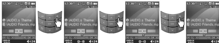
1. During music playback, press the button to set the start of the section to repeat. icon will appear on the bottom of the status bar.
