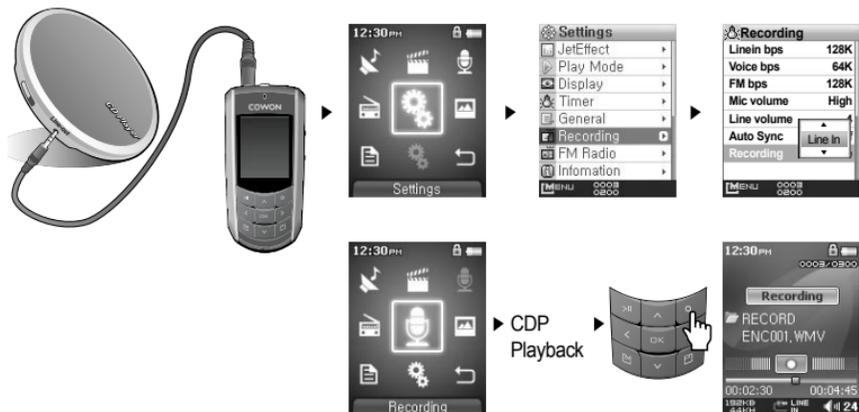
1. Use the Line-In cable to connect the headphone jack of your audio source device with the Line-In jack of iAUDIO F2.
