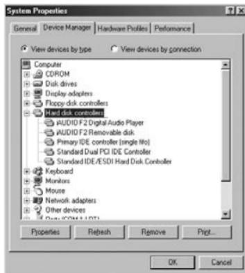
8. Click the "Finish" button to complete the driver installation. The newly added drive can be seen in Device Manager or Explorer.
