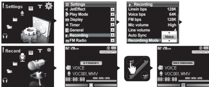
1. Make sure that the recording mode is set to Voice in Settings – Recording- Recording Mode menu.
