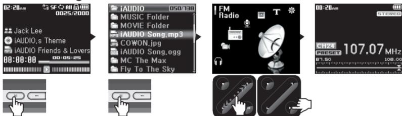
iAUDIO 7 has 7 modes of operation (Music, Video, FM Radio, Record, Picture, Text, USB Host) and Settings menu. To switch between these modes, Press "MENU" button twice. Mode selection screen will appear. (Pressing the "MENU" button once will switch the display to current folder view.)
