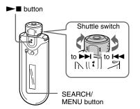
1 Press and hold the SEARCH/ MENU button for half a second while the audio player is stopped or receiving an FM signal.
